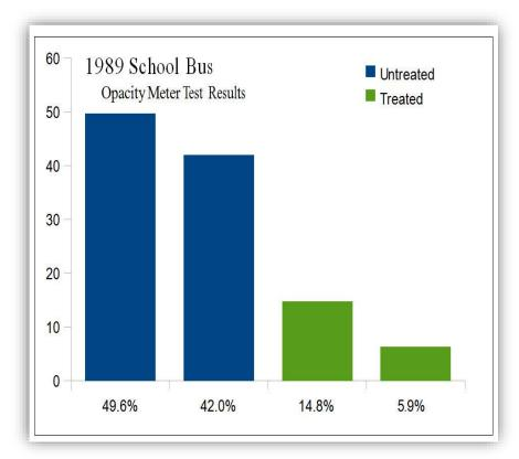
The opacity readings from the two baselines snap tests on February 13, 2009 were **49.6%** and **42.0%**, snap
