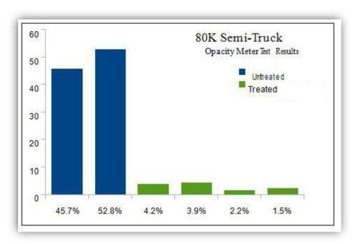
The opacity readings after using the CatX were 4.2% and final density of 1.5%. Diesel smoke was almost completely eliminated and fuel efficiency was improved.
